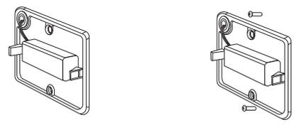
Align the main body with the bottom shell for assembly, and then tighten the screws on the left and right sides in turn.
